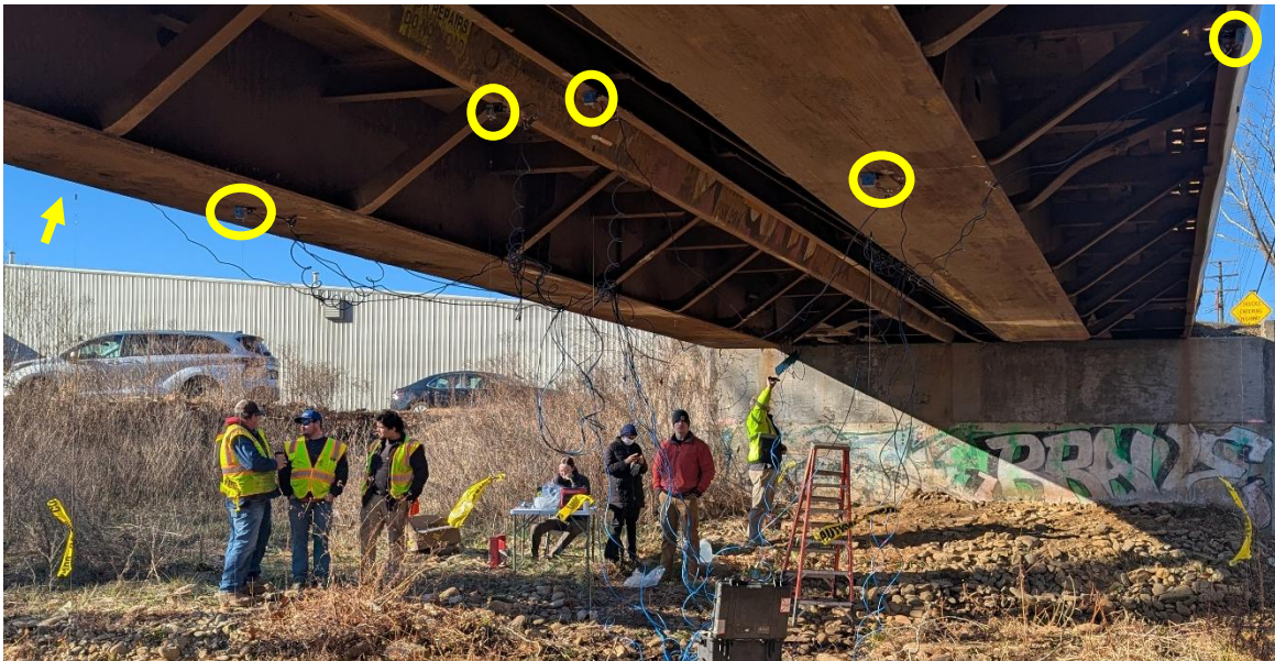
Figure 9. Measurement locations at the structure midspan (yellow circles and one yellow arrow)
