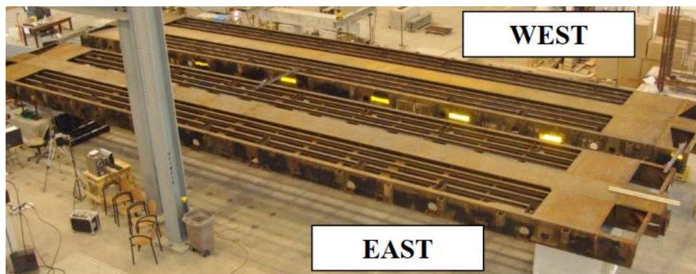
Figure 5. Significant Previous Experiments at Purdue University on Two Adjacent RRFCs, Prior to Adding a Composite Concrete Deck. Reproduced from the 2015 Purdue Phase III Final Report. Note the 47' support span, supports inset at the truck mounts, and lack of an integral deck.
